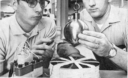
ELECTROMAGNETIC SYSTEM to keep pendulum swinging is checked in the electronic apprentice shop by (I to r) Clifford C. Condit and Joseph E. Brown, both electronics apprentices who graduated recently. They developed the system to keep the pendulum in Sandia's Sphere of Science swinging for long periods of time.
